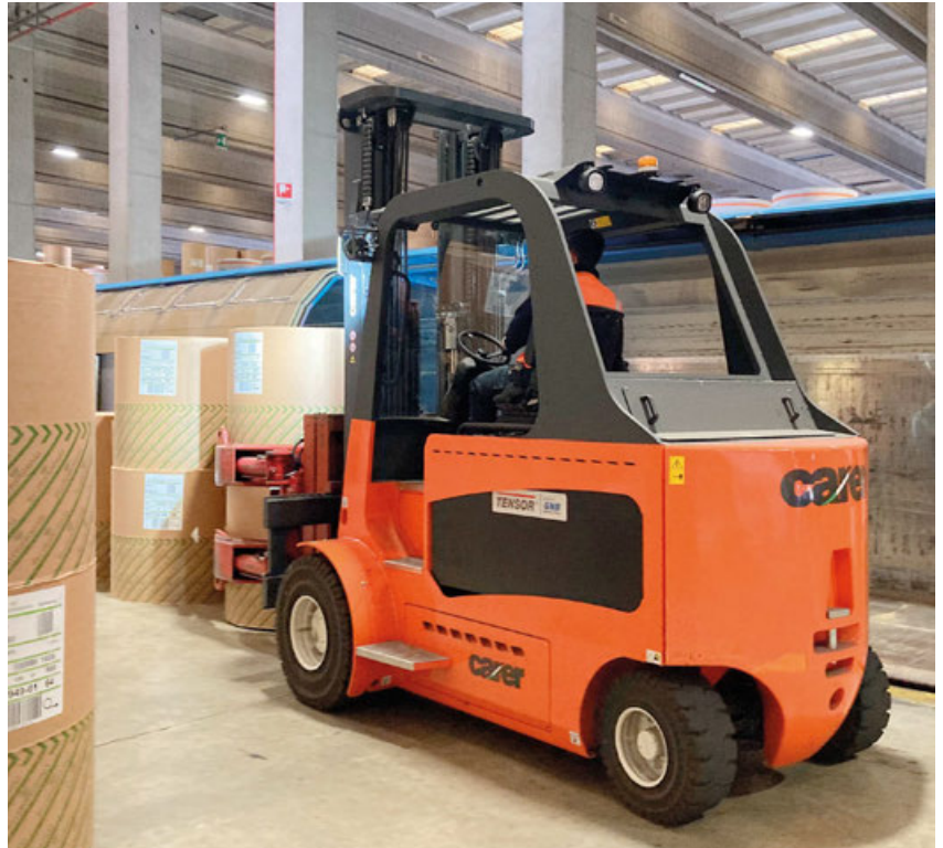
▲ Carer Z80H2 is picking up paper rolls.
