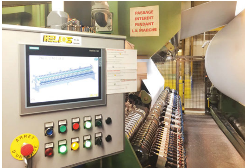
▲HELIOS - HMI panel control for 43 cutting unit.
