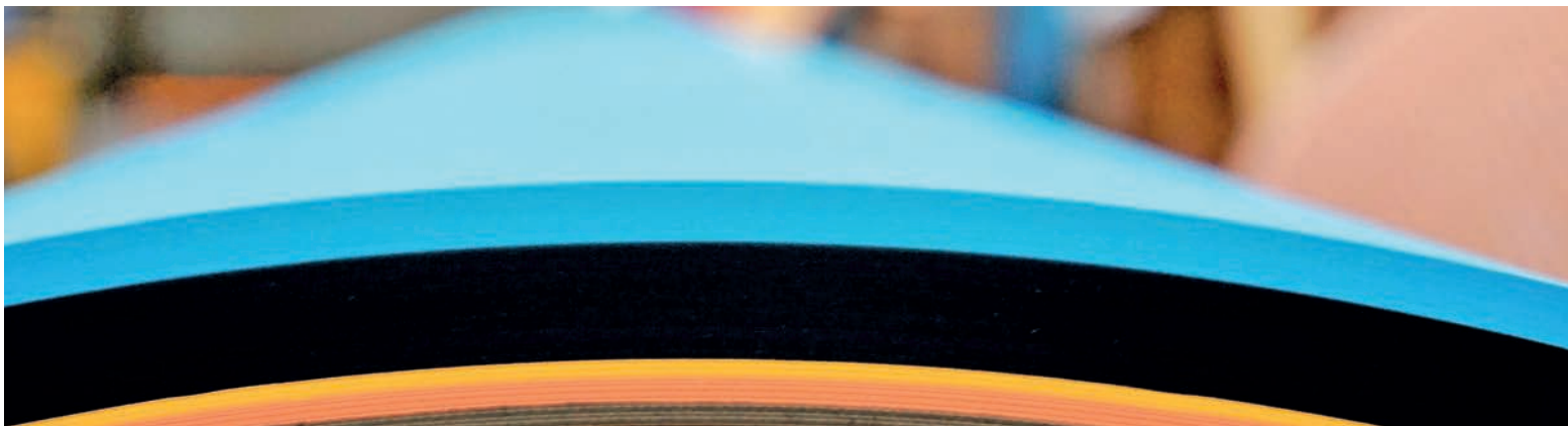
▲ Profile view of a Maxidry cover where the Triplex - Multilayer confection can be noted.
