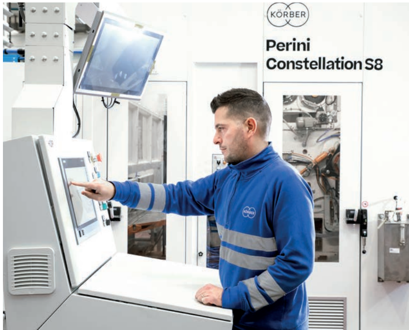
▼ Operators govern the machine's start-up from the external HMI panel.
