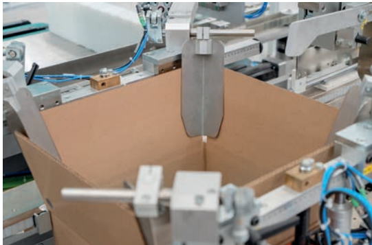
◀ Fully servo-driven OMET case packer.
