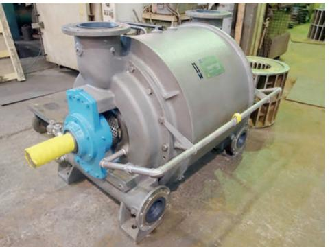
▲ VAKUO CNN pump with dismountable bearing brackets. VAKUO vacuum pumps are interchangeable with other brands, they are "bolt-on" replacements (same performances, same dimensions) but offer many features/advantages like for example the removable bearing brackets.
