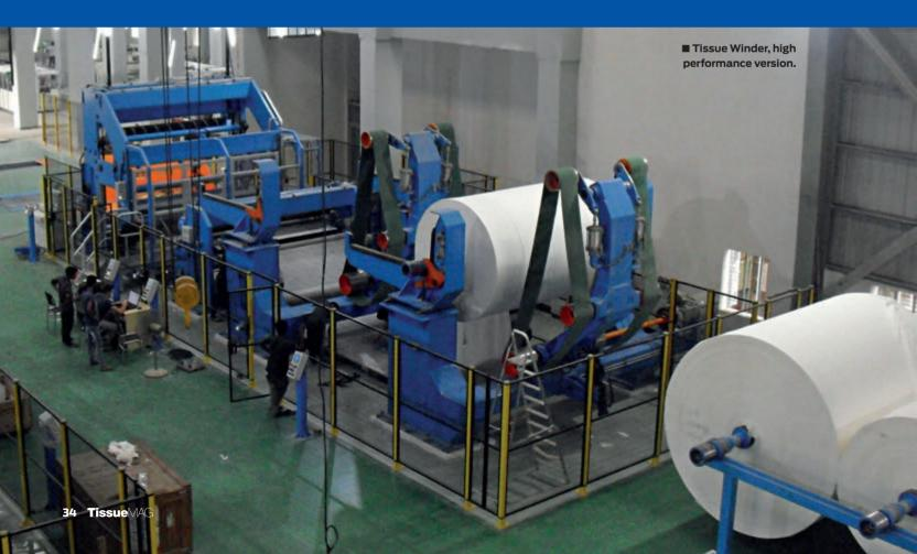
When winding tissue there are many factors that limit the winders operating speed. On "conventional" tissue products the main limiting factors are: paper width, number of plies, diameter of cores at wind-up, number of slitters into operation.
