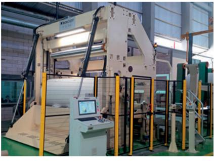
▲ Tissue Winder with automatic web tension control at unwinder.
