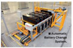
charge is low, the vehicle, when finished the mission, goes automatically to the battery charging station. Change happens in a few minutes. There also exist models in which re-charge takes place automatically in a partial re-charge station. In this case the vehicle dedicates all block times to auto-recharge of the batteries, without operator intervention. It allows for continuous operation.
