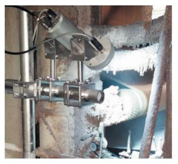
▲ Web Monitoring Systems have become more intuitive allowing operators to quickly and efficiently find the root cause, or origin, of their break causing defect or other quality issue.
