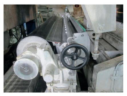
▲ Fig: 3. Felt Roll Doctor complete with shower pipe and internal cleaning brush.
