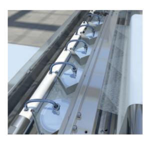
▲ W+D FLOWTOS may be equipped with the WEKO rotor damping system to apply liquids.
