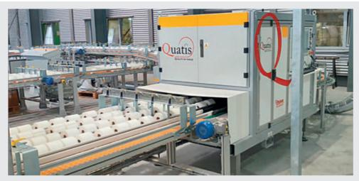
▲ Quatis machine for the inspection of rolls.
